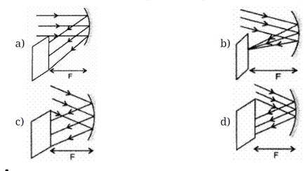
75.Four students A, B , C and D carried out measurement of focal length of a concave mirror as 1 shown in the following four diagrams.
